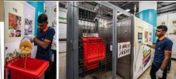
The food waste composting process is fully automatic. The waste just needs to be loaded onto the Eco Digester's conveyor lift and it will be processed within 24 hours.
